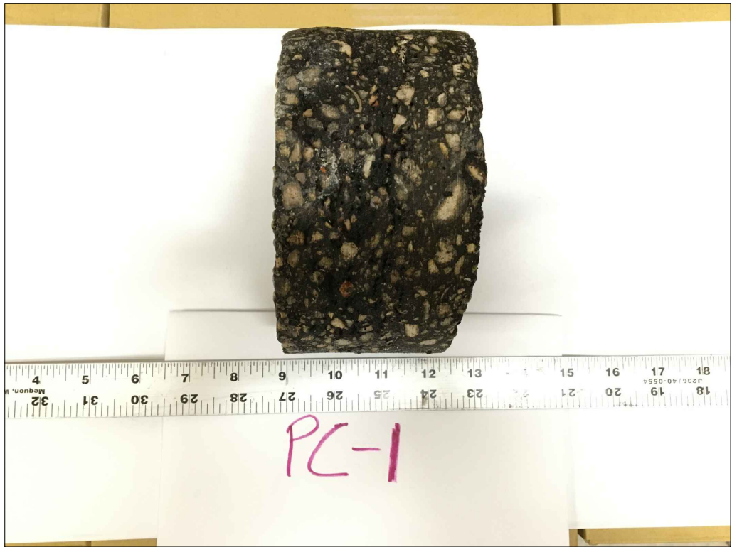
3.0 INCHES THICK ASPHALT
